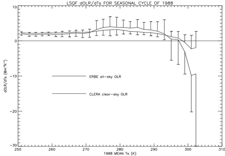
Figure 6.11: Least squares fit  $dOLR/dT_s$  for CLERA clear-sky and ERBE all-sky OLR with mean  $T_s$  for the seasonal cycle of 1988. Error bars denote one standard deviation of values for each  $T_s$  bin and are plotted either above or below the mean value only for reasons of clarity. The bars are displayed to highlight the statistical scatter associated with the calculated sensitivity rather than the physical uncertainty associated with the models and data.
