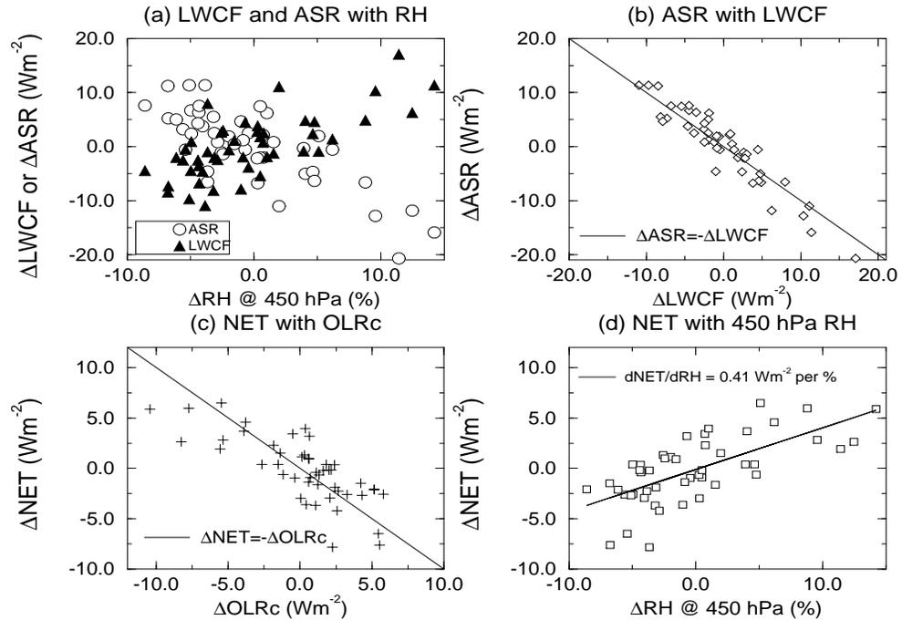
Figure 6.22: Relationships between interannual monthly anomalies of the top of atmosphere irradiance and RH for the northern sub-tropical Pacific ( $170$  to  $210^\circ$  E and  $10$  to  $25^\circ$  N) over the period February 1985 to January 1989. (a) LWCF (triangles) and ASR (Circles) with ERA 450 hPa RH. (b) ERBE ASR with CLERA-ERBE inferred LWCF. (c) ERBE net downward irradiance with CLERA clear-sky OLR. (d) ERBE net downward irradiance with ERA 450 hPa RH.
