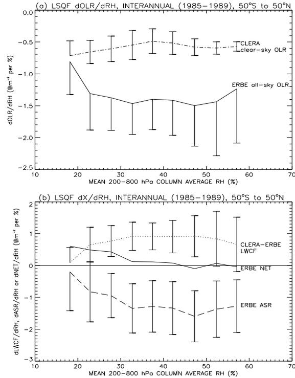
Figure 6.20: *LSQF all-sky and clear-sky  $dOLR/dRH$  (a), and  $dLWCF/dRH$ ,  $dASR/dRH$  and  $dNET/dRH$  (b) for the interannual time-scale for 5% bins of mean  $RH$ . Units are  $Wm^{-2}$  per %. Vertical error bars denote one standard deviation about the mean sensitivity calculated for each  $RH$  bin and are displayed to highlight the statistical scatter associated with each calculated sensitivity rather than the physical uncertainty associated with the models and data.*
