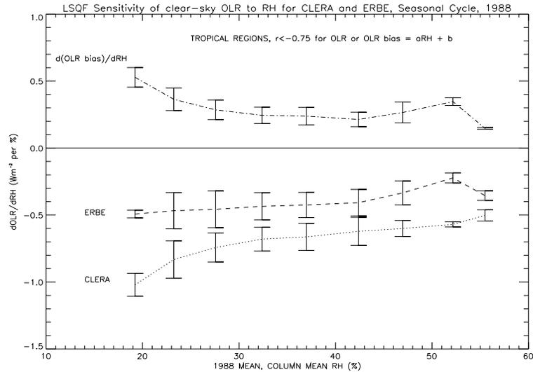
Figure 6.8: *LSQF*  $dOLR_c/dRH$  for CLERA, ERBE and the ERBE-CLERA  $OLR_c$  bias ( $-\delta OLRC$ ) for 5% bins of RH for the seasonal cycle of 1988. One standard deviation about the mean is plotted for each bin as an error bar and are displayed to highlight the statistical scatter associated with the calculated sensitivity rather than the physical uncertainty associated with the models and data. Only regions for which  $r < -0.75$  for all three regressions are considered.
